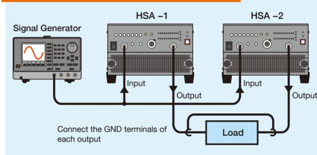
The output of the signal generator is divided and input to HSA -1 and. HSA -2 has a reverse phase output towards HSA -1.
