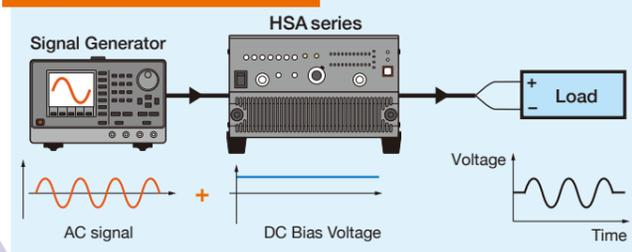
Set the rated DC voltage of the load with the DC bias of the HSA and superimpose the AC voltage output from the signal generator.
