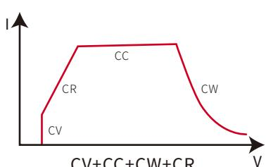
CV+CC+CW+CR mode can be applied to test lithium-ion battery charger, to gain complete V-I charging curve.In addition, when protection circuit of DUT is damaged, it can auto switch to avoid damage.
