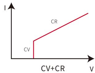
CV+CR mode can be applied to simulate LED light, test LED power, LED current ripple parameters.
