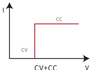
CV+CC mode can be applied to load simulate battery, test charging station or car charger, the maximum loading current is limited,when the CV is working.
