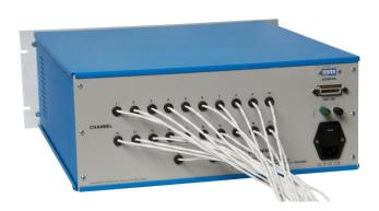
The B Series features four-conductor Teflon Cable inputs with 2 four-conductor Teflon Cable outputs attached directly to the relay boards reducing the number of contacts. Each B series scanner comes with a 2 meter lead. As an option, the leads can be extended to 3 or 4 meters.
