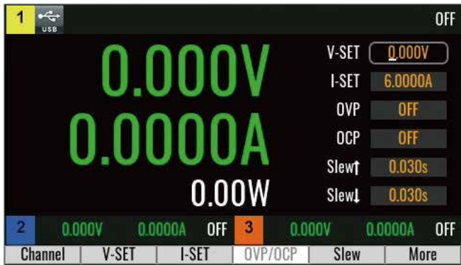
Single-Channel Meter Interface and Quick Setup Interface
